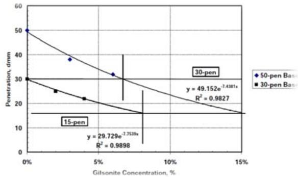
Adding Natural Bitumen (“Gilsonite-Like”) as a regulator to Asphalt increases its quality. For example according to the R & B (ball and ring) test and experiment, the soft point of Asphalt after adding Natural Bitumen (“Gilsonite-Like”) reaches 149<sup>0C</sup> from 139<sup>0C</sup> and this shows that Asphalt softens at a higher temperature and can be used in high temperature zones.
